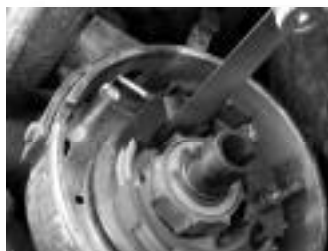
Distributor with dust cap removed and feeler gauge inserted
