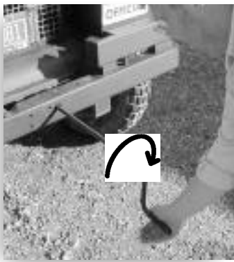
Long FC 101 crank handle used to help illustrate correct hand grip & rotation in a clockwise motion. Series handle will be shorter.
